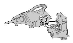
**4** Adjust the adaptor to hold the base unit, then push it in the direction of the arrow until it clicks into place.
