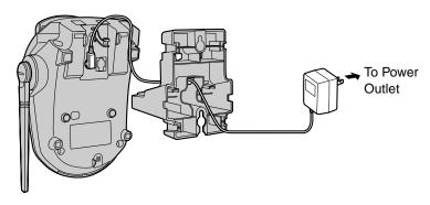
**2** Tuck the telephone line cord inside the wall mounting adaptor (1). Connect the telephone line cord (2) to the unit.
